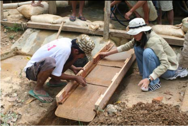
A local miner and Lestari's trainer testing sluice box in Tanoyan, Sulawesi.
